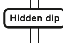
Other danger; plate indicates nature of danger
