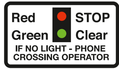
Miniature warning lights at level crossings
