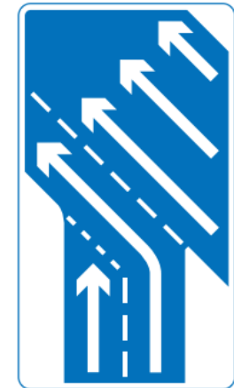
Traffic in right hand lane of slip road joining the main carriageway has priority over left hand lane
