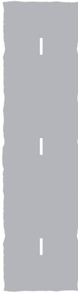
Lane line separating traffic travelling in the same direction (single or dual carriageway road)
