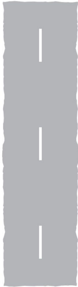
Centre line on a single carriageway road
