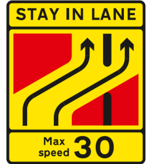
One lane crossover at contraflow road works
